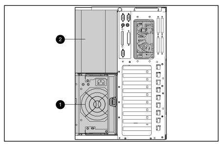
Figure 2-33. Power supply bay configuration
